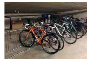
Racks are wheel benders (Photo: Alta Planning + Design)
